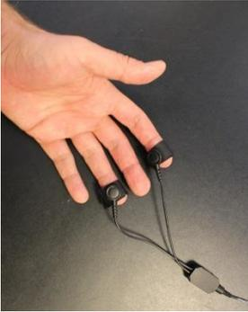
Cleaning: After the use, clean the sensor using a water and mild soap with dampened cloth.
