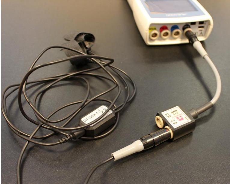
Image 1: GSR-sensor connected to ME6000 through datalocker on channel 1
